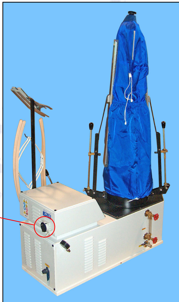
Figure chap. 7.2 "Main switch"
